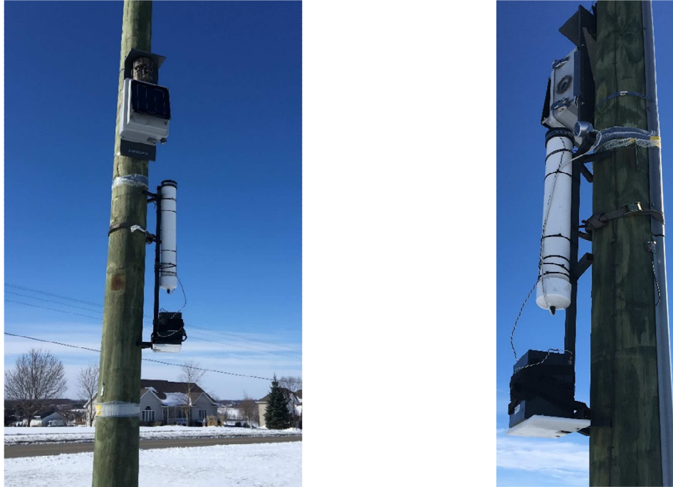
Figure 3.15 Front and side views of the Moultrie and IFC web-cameras
