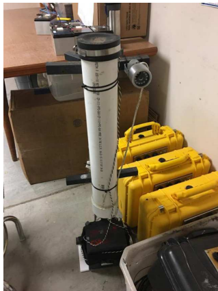
Figure 3.14 a) IFC webcam; b) Sample image taken from IFC webcam
