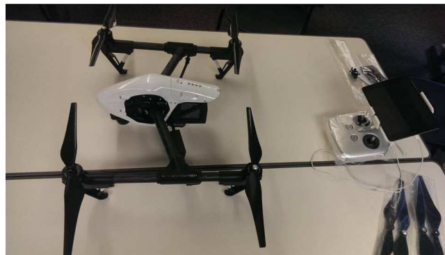
Figure 3.11 DJI Inspire 1 unmanned aerial vehicles
