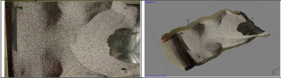
Figure 5.6 Comparison between Agisoft software 3-D maps output and physical measurements
