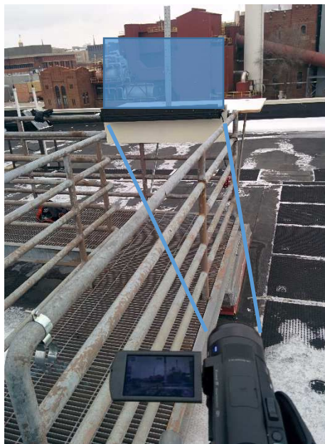
Figure 4.5 Sketch showing the vertical plane in which the movement of the snowflakes was visualized
